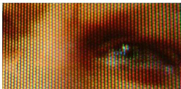
By Martin Howard [CC BY 2.0 ( https://creativecommons.org/licenses/by/2.0 ) or CC BY 2.0 ( https://creativecommons.org/licenses/by/2.0 )], via Wikimedia Commons; Close-up of an analog television screen, displaying the trichromatic composition of the image.
