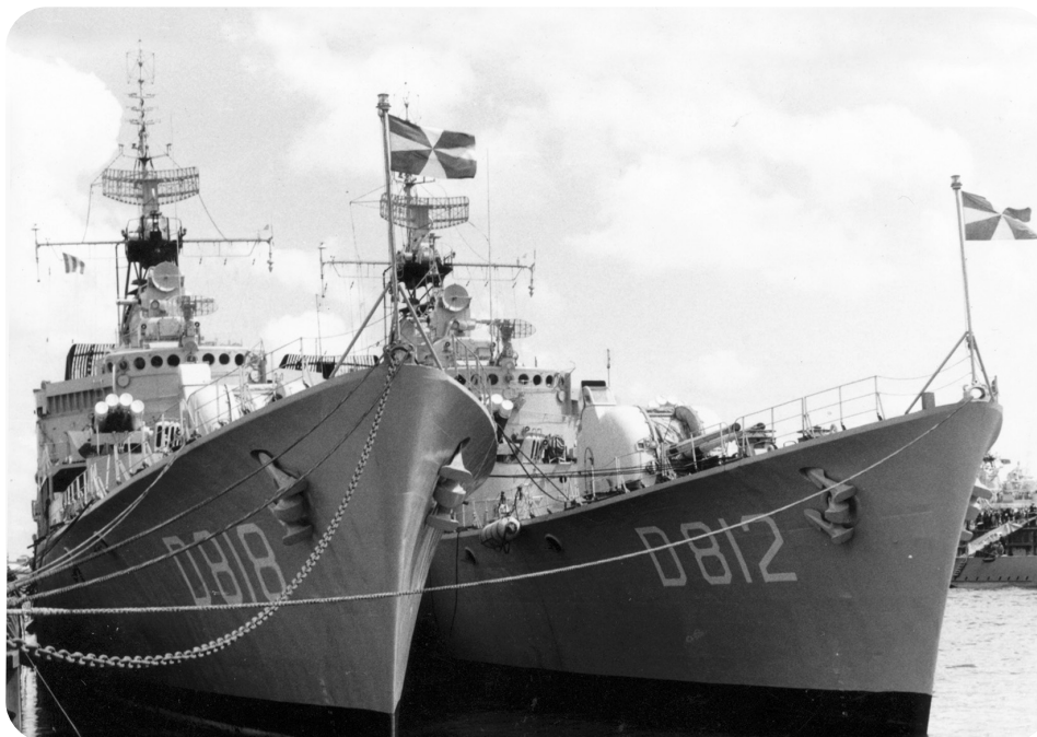
Trials of Drenthe. Note the absence of air warning (LW-02) radar antenna.
