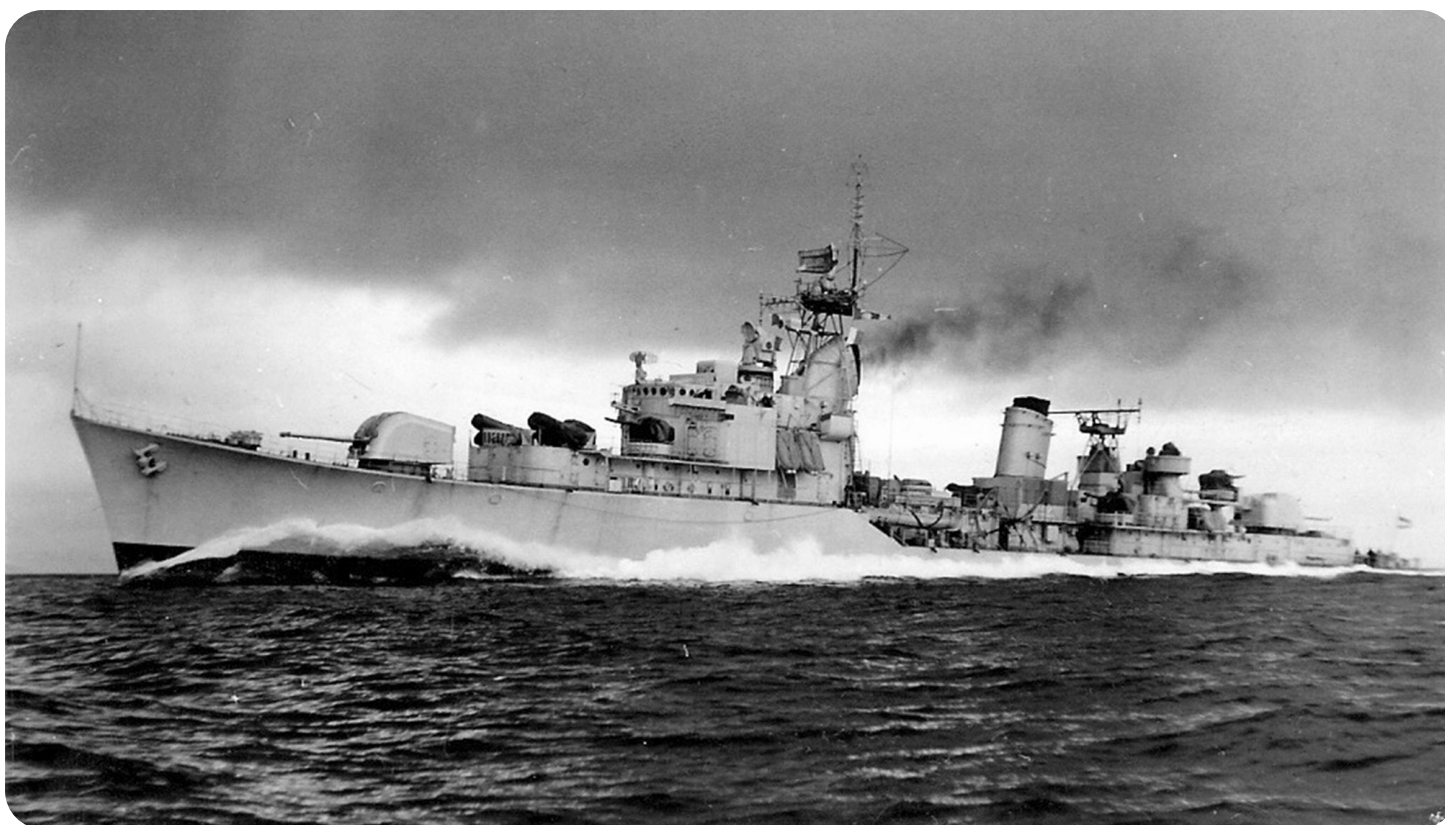
Trials of Drenthe. Note the absence of air warning (LW-02) radar antenna.
