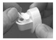
Snap the white membrane onto the yellow valve until the membrane lies flat against the valve.
