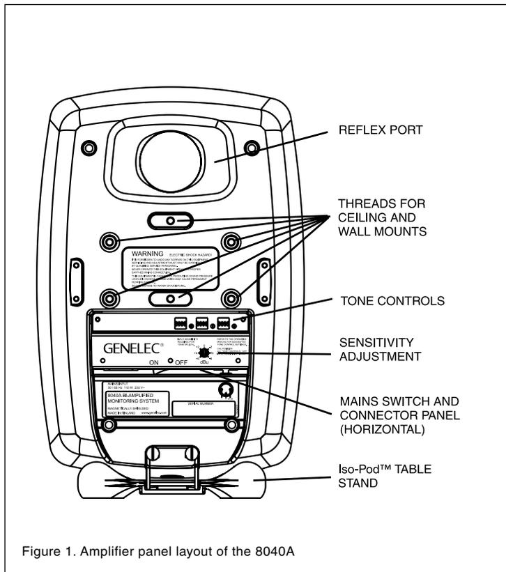
Figure 1. Amplifier panel layout of the 8040A
