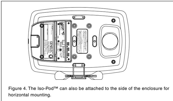
Figure 4. The Iso-Pod™ can also be attached to the side of the enclosure for horizontal mounting.
