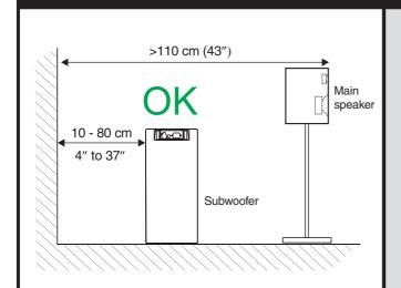
Positioning too far from the wall may cause a loss in low frequency response
