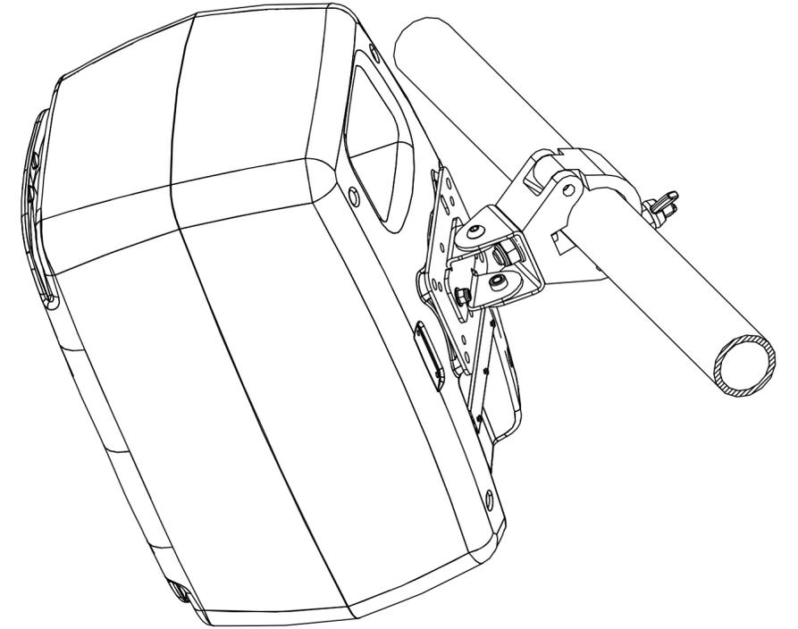
Mounting on a vertically frame tube (Ø48-Ø51mm)
