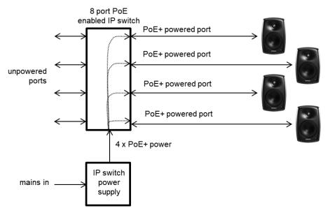
Example of powering the 4420A with a PoE+ enabled IP switch. With this method, the power budget available for all outputs connected to the IP switch must enable each 4420A to run at full PoE+ power. For 4 loudspeakers, the power supply must support 4 x PoE+ power level.
