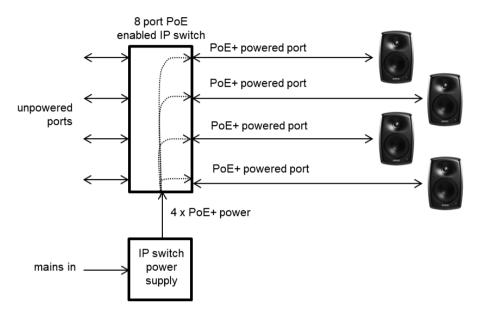
Example of powering the 4420A with a PoE+ enabled IP switch. With this method, the power budget available for all outputs connected to the IP switch must enable each 4420A to run at full PoE+ power. For 4 loudspeakers, the power supply must support  $4 \times PoE+$  power level.
