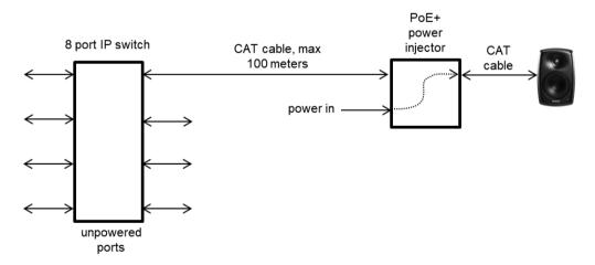
Example of powering the 4420A with a PoE+ power injector. This method enables the use of standard non-PoE IP switches. Each power injector must support full PoE+ power level into the device.
