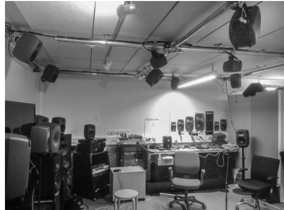
Figure 1c. Side view to the 22.2 immersive speaker layout.
