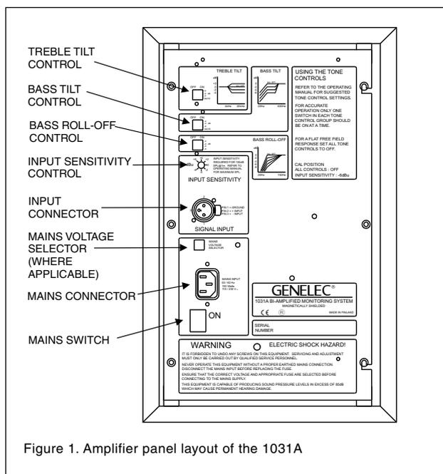
Figure 1. Amplifier panel layout of the 1031A
