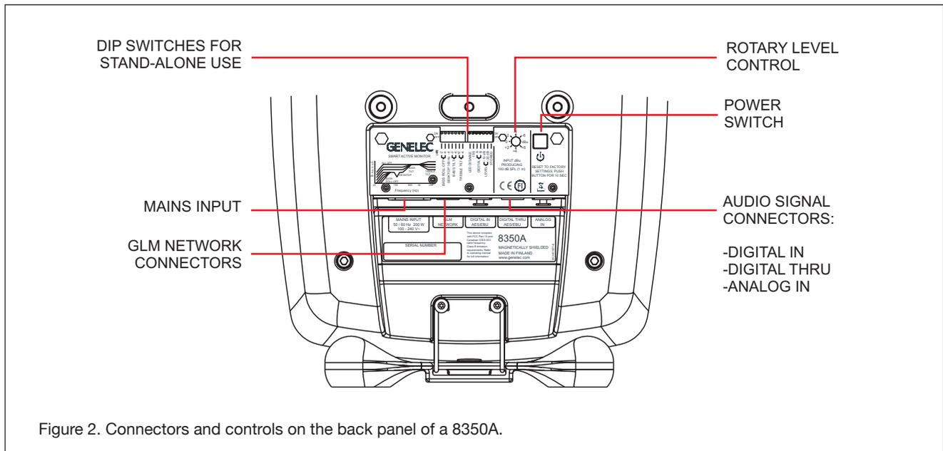
Figure 2. Connectors and controls on the back panel of a 8350A.
