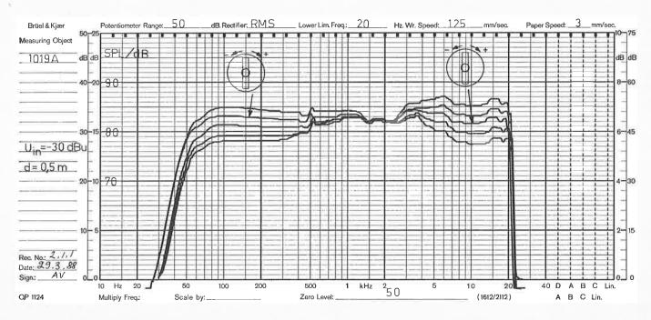
Effect of control settings measured in free field conditions:
