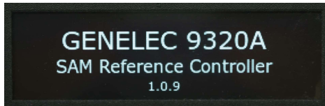
Fig. 26. The start-up splash screen shows the firmware version number on the last line.
