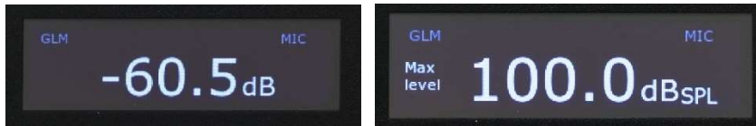
Fig. 6. Relative level display (left), absolute SPL level display (right).
