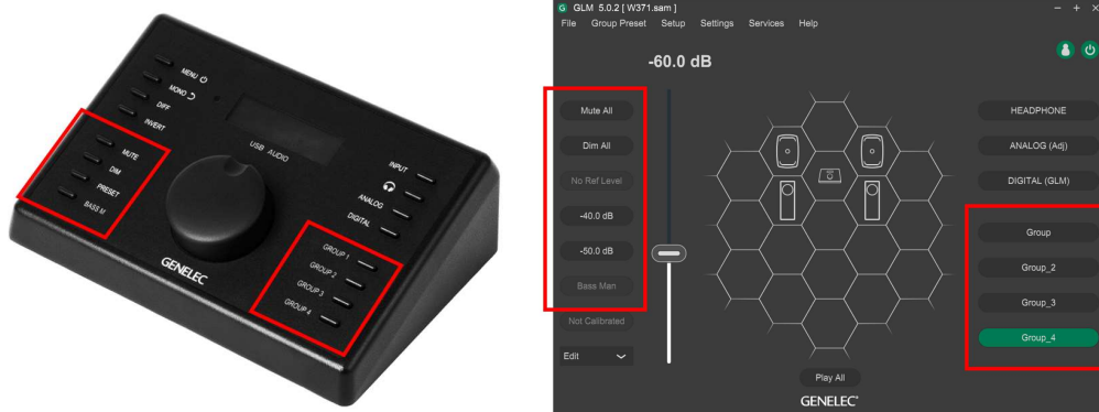
Fig. 7. The matching controls in the 9320 (left) GLM software (right).
