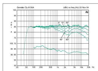
Figure 3: The upper curve group shows the horizontal directivity characteristics of the 8130A measured at 1 m. The lower curve shows the systems power response.
