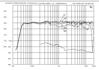
Figure 4. The upper curve group shows the horizontal directivity characteristics of the 1032A in vertical configuration measured at 1 m. The lower curve is a 1/3 octave band power response, measured in an IEC approved reverberation chamber.
