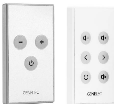
Figure 48. Two wireless remote controllers to use with GLM
