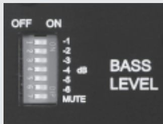
Calibrated 'Level' switch. MUTE disconnects the channel for testing.
