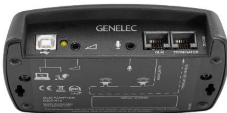
Figure 59. GLM Network Adapter connections from left to right: USB to computer or to USB power supply, hardware level controller input, GLM Measurement Microphone input, GLM Network and Terminator connectors.
