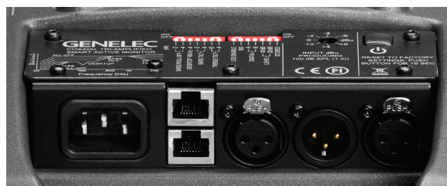
Figure 3. Connector panel detail.
