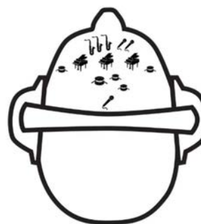
Virtual sound sources appear inside the listener's head with standard headphone listening
