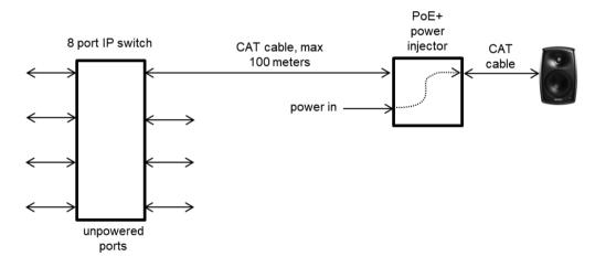
Example of powering the 4430A with a PoE+ power injector. This method enables the use of standard non-PoE IP switches. Each power injector must support full PoE+ power level into the device.
