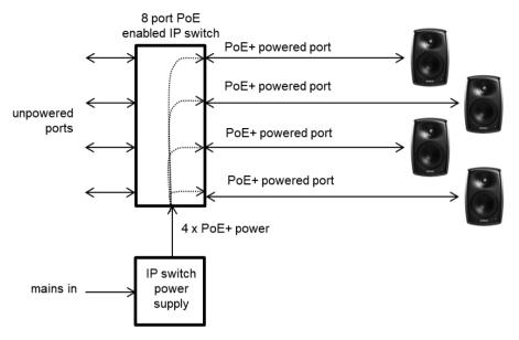
Example of powering the 4430A with a PoE+ enabled IP switch. With this method, the power budget available for all outputs connected to the IP switch must enable each 4430A to run at full PoE+ power. For 4 loudspeakers, the power supply must support 4 x PoE+ power level.
