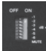
Calibrated 'Level' switch. MUTE disconnects the channel for testing.
