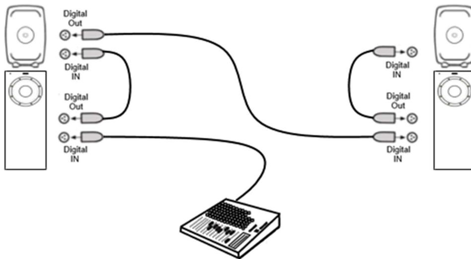
Figure 7. Digital stereo adaptive woofer system cabling.
