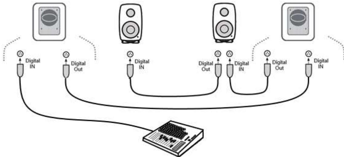
Figure 46. Dual subwoofers with the AES/EBU signal.
