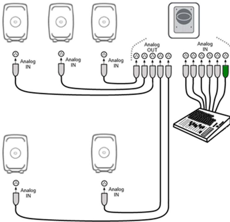
Figure 5. An example of analog 5.1 system cabling
