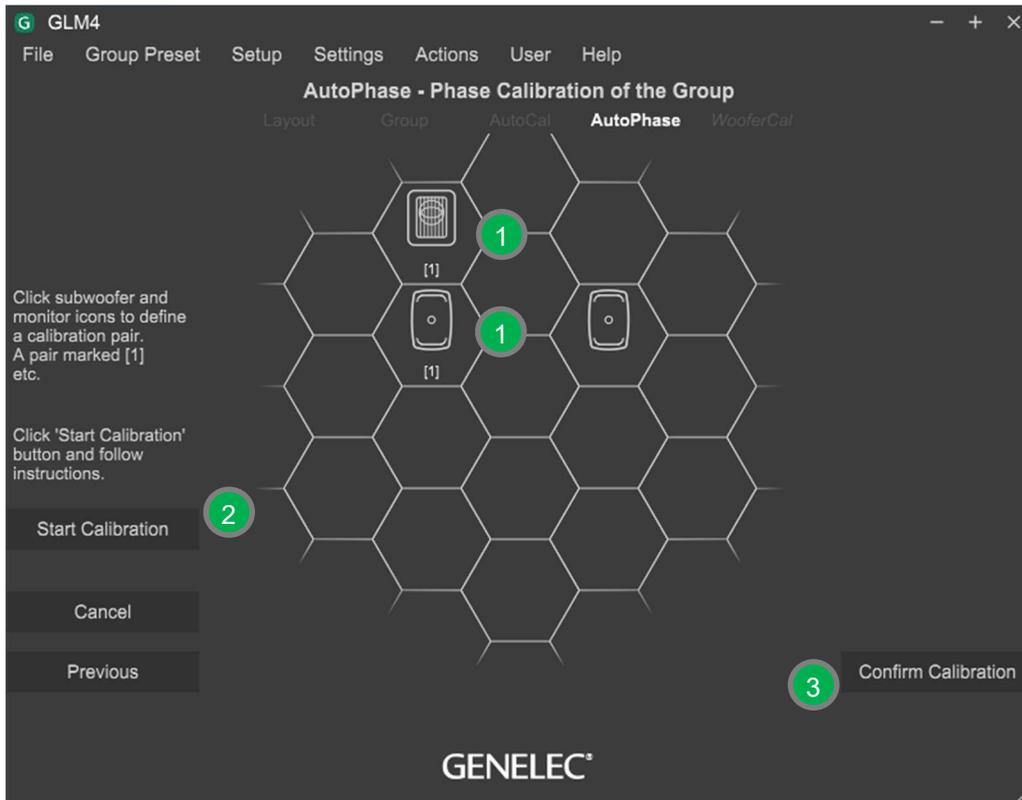
Figure 19. Steps in running the AutoPhase automatic phase calibration process
