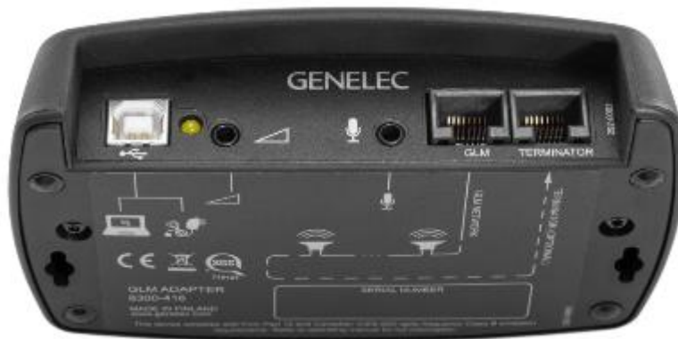
Figure 47. GLM Network Adapter connections from left to right, USB to computer or to USB power supply, hardware level controller input, GLM measurement microphone input, GLM network and terminator connectors.
