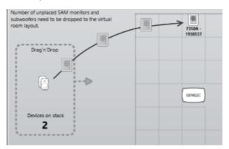
Figure 14. Drag and drop the monitor icons onto the layout grid to build a system layout
