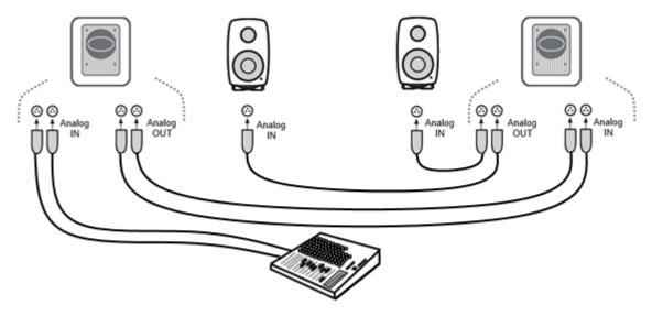
Figure 48. Dual subwoofers with the analogue signal.
