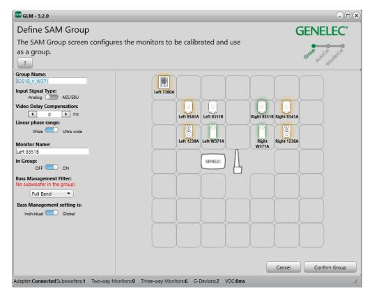
Figure 32. Common settings for a SAM group are presented on the left side of the SAM group definition display.
