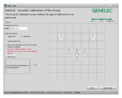
Figure 34. Microphone layout for MultiPoint calibration
