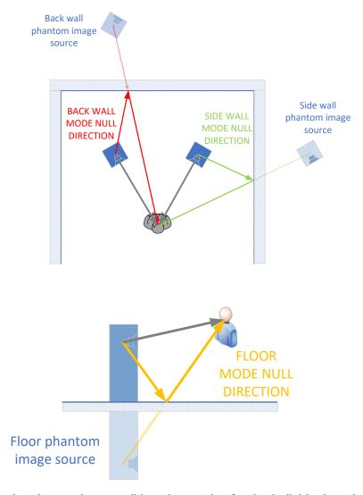
Figure 22. Diagram showing the maximum null location angles for the individual modes\*
