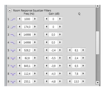
Figure 38. Room response equalizer controls
