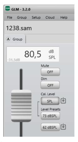
Figure 27. Calibrated SPL level.
