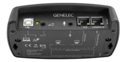
Figure 43. GLM Network Adapter connections from left to right, USB to computer or to USB power supply, hardware level controller input, GLM measurement microphone input, GLM network and terminator connectors.
