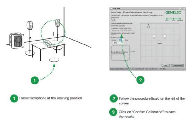
Figure 20. Steps in running the AutoPhase automatic phase calibration process
