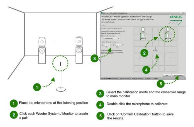
Figure 21. Adaptive woofer system calibration.
