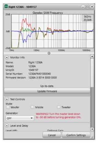
Figure 36. Example of the acoustical calibration editor window
