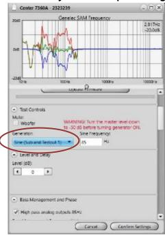
4. Using the mic SPL reading slowly change **Phase setting** using the < or > keys. We suggest you start at -180 then click > stopping at -135, -90, -45, 00, +45, +90, +135, +180 and then noting which setting is the loudest SPL on the mic. Do this slowly (about 4 seconds secs) as the mic uses a slow update rate. Then Choose Confirm Settings.
