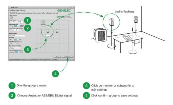
Figure 18. Group definition window; the monitors with a green halo is active; monitors with a yellow halo are not part of the active group
