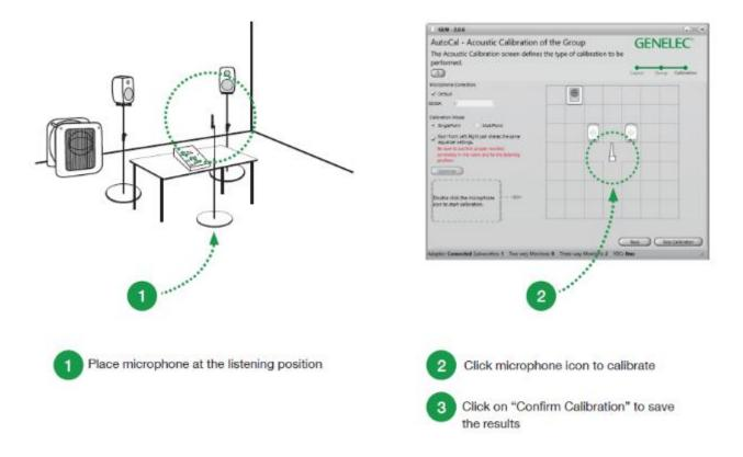
Figure 19. Steps in running the AutoCal automatic system calibration process
