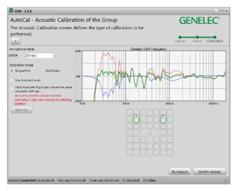
Figure 35. Reviewing the corrections by clicking on the monitor and subwoofer icons
