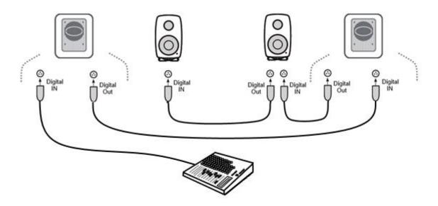
Figure 49. Dual subwoofers with the AES/EBU signal.
