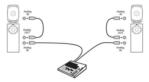
Figure 3. Analog stereo woofer system cabling.
