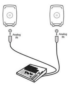
Figure 2. Analog stereo cabling.
