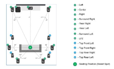
Defining a system layout in GLM: Start by dragging monitors/subwoofers from the Drag'n'Drop box to the grid. Each monitor and subwoofer plays an ID tone when dragged and that helps to identify which monitor is handled. For example, when dragging a subwoofer it plays a sine tone and can be placed to the grid. Next page shows an example where each monitor is placed to match an Atmos layout. Note that monitors may not appear in the same order as in these examples.
