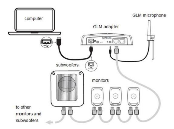
Figure 12. Connections of GLM control network, measurement microphone, and computer
