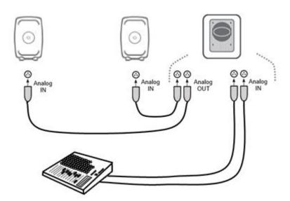
Figure 4. Analog stereo cabling with a subwoofer
