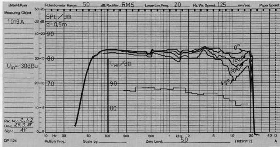
Figure 6. 1019A Directivity characteristic and power response
