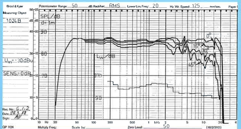
Directional characteristics and total radiated acoustic power response (measured in reverberation chamber at 1/3 octave bands).
