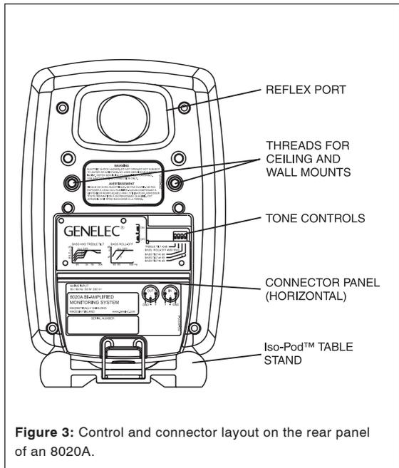
**Figure 3:** Control and connector layout on the rear panel of an 8020A.
