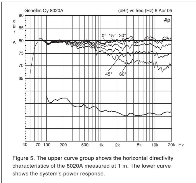
Figure 5. The upper curve group shows the horizontal directivity characteristics of the 8020A measured at 1 m. The lower curve shows the system's power response.
