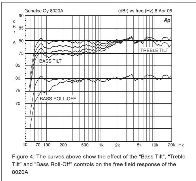
Figure 4. The curves above show the effect of the “Bass Tilt”, “Treble Tilt” and “Bass Roll-Off” controls on the free field response of the 8020A
