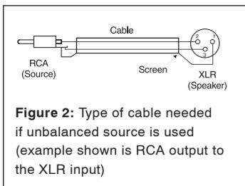
**Figure 2:** Type of cable needed if unbalanced source is used (example shown is RCA output to the XLR input)
