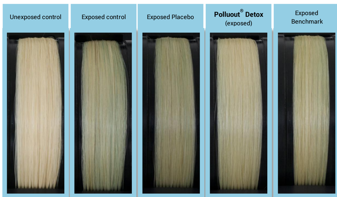
Figure 16: Colorimetry results (Delta a) after exposure in the \text{CuSO}_4 solution, and after 5 shampoo treatments.
