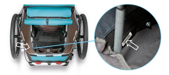
When you are standing behind the vehicle, you can find the serial number at the bottom of the black frame on the left side (with respect to the direction of travel). You will see a white sticker with a barcode and above the serial number.
