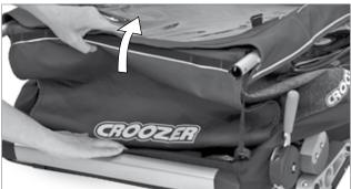
Holding the upper frame tube in the raised position, pull the seat frame slowly and carefully back and towards you until the locking pins (5) of both locking mechanisms (4) engage with audible clicks in the holes (6) of the frame tubes.
