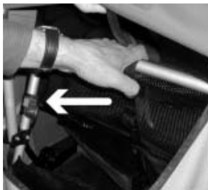
Then put your hand into the Croozer and pull the seat handle back.
