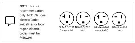
Your equipment comes with a power cable that meets your local electrical code requirements along with the equipment. Precor treadmills must be connected to a 20 amp individual branch circuit that can be shared only with one PVS.
