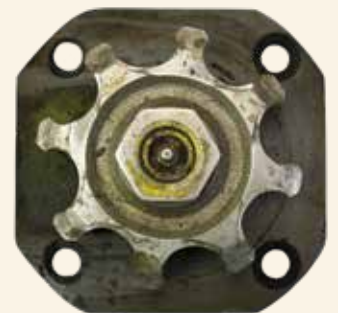
SPROCKET WEAR WITH OFF-BRAND GATHERING CHAINS
