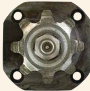
SPROCKET WEAR WITH DRAGO GATHERING CHAINS
