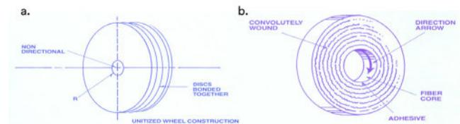
**Figure 1:** Construction of a) unitized and b) convolute wheels.
