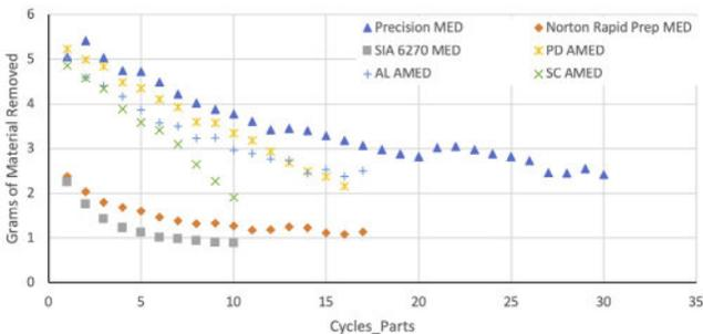
**Figure 7:** The amount (grams) of material cut during each one-minute cycle is illustrated for Scotch-Brite™ Precision, AL, PD and SC. Scotch-Brite™ products are compared to Norton Rapid Prep and SIA 6270 discs.
