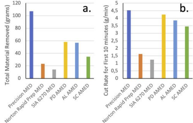
**Figure 6:** Shows a) the total amount of material (aluminum) removed at the disc's end of life and b) the average cut-rate per minute for each disc type in the first 10 minutes of testing for Scotch-Brite™ and leading competitors.
