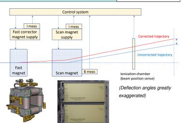
Control scheme (one axis shown) and a two-axis MN60 ferrite corrector magnet with pole length 10 cm, pole gaps 7 cm, calculated self inductance 76  $\mu$ H and resistance 10 m $\Omega$  per axis. Deflection angle for 230 MeV protons is 2.2 mrad. The magnet is designed to be powered by one IECO PA400-350 four-quadrant supply per axis with current control bandwidth >10 kHz, DC current up to 140 A, voltage compliance 350 V.
