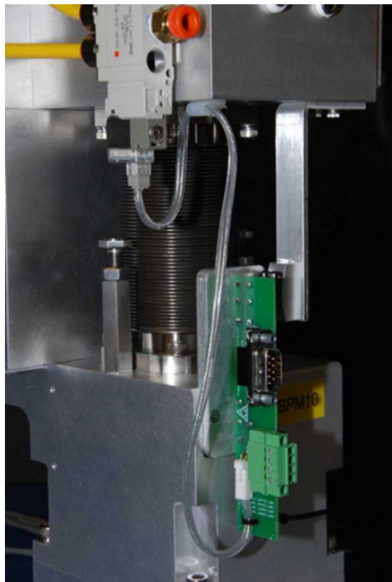
Figure 9. High flex cable connecting the actuator control connector to the solenoid valve.
