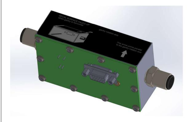
Shown with 1/4" NPT to 3/8" push-fit tube adaptors as supplied. For gantry systems, top face should be parallel to ground when gantry angle is 90 degrees. Arrow should be parallel to rotation axis.
