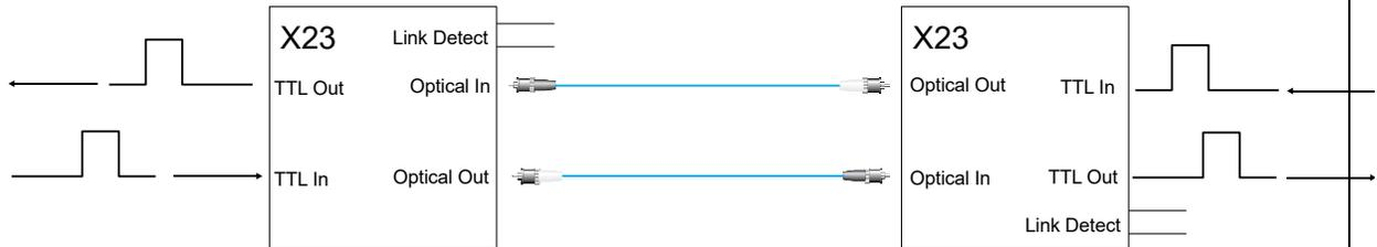
The bidirectional configuration transmits independent level information between two systems. At each location, the link detect relay indicates that the receiving optical link is intact.
