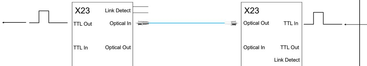
In many applications, only a single link is required. The link detect relay indicates that the receiving optical link is intact.
