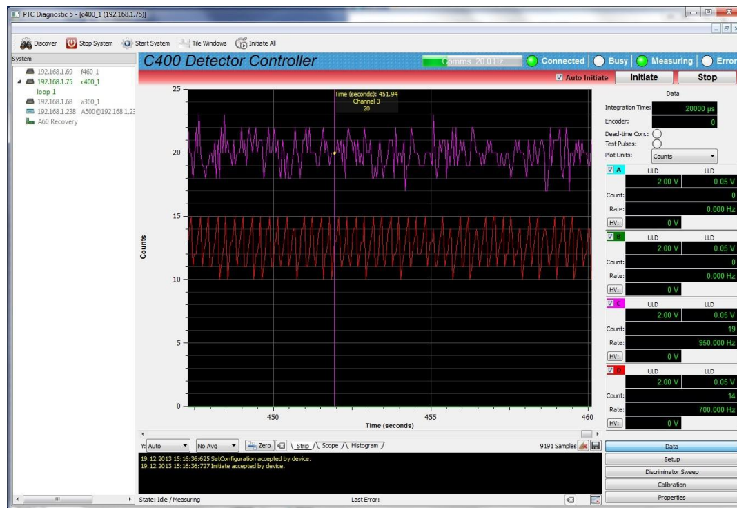
Figure 14. Strip chart data display showing cursor. The scope display looks similar.
