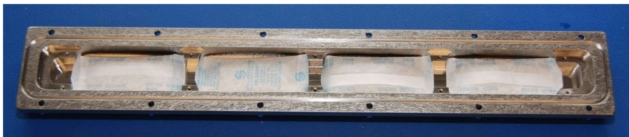
Figure 25. Installation of the desiccant sacs
