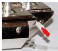
Figure 22. Plugging flow gas port for operation with dry atmospheric air
