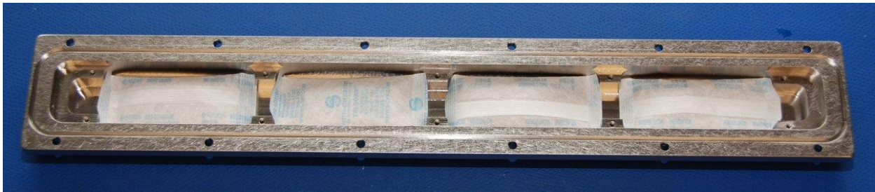
Figure 25. Installation of the desiccant sacs
