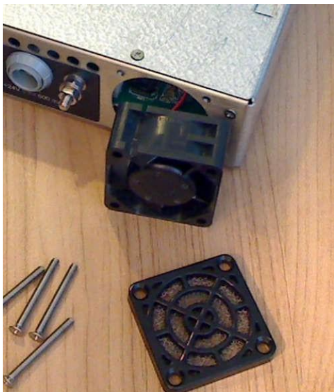
Figure 78. Fan filter removal
