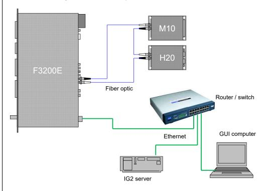
Any EPICS client that need to communicate with IG2 must be in the same network broadcast domain as IG2. The IG2 server can run on the GUI computer or on a separate server.
