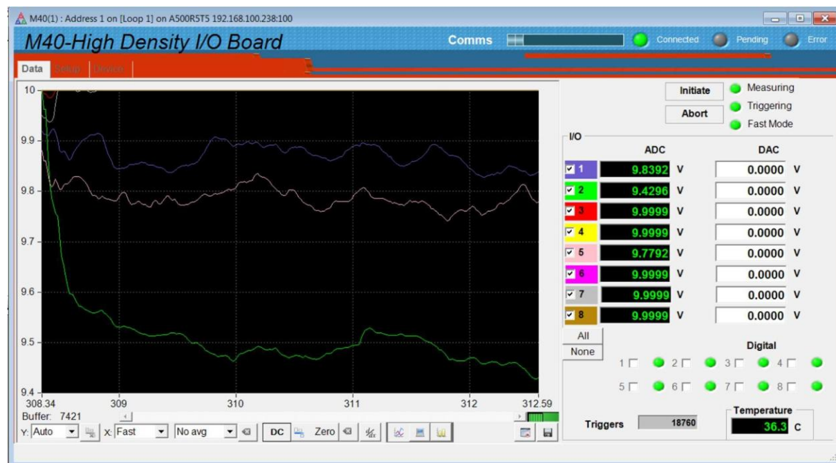
Figure 10. Data tab: M40 running with default settings, showing autoscaled background noise on the inputs.
