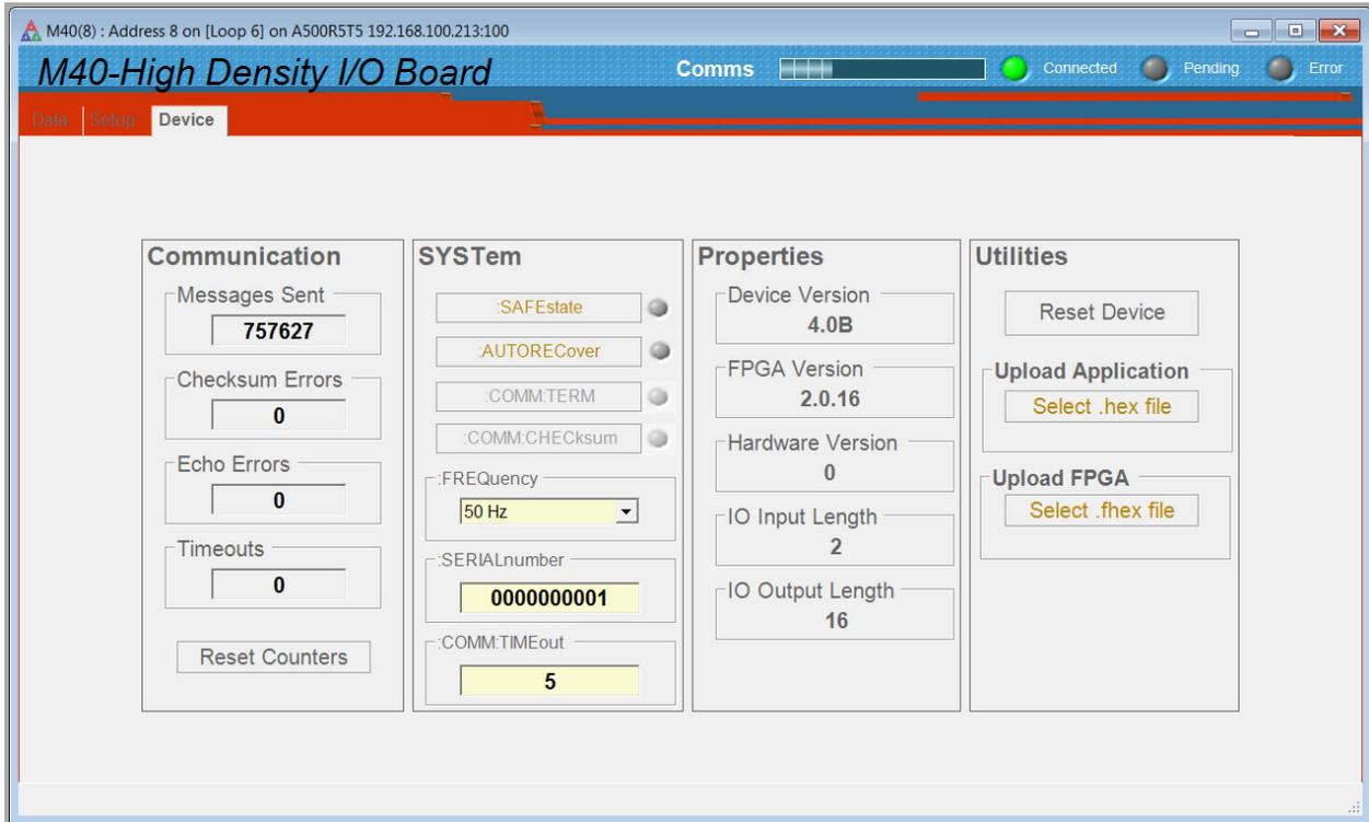
Figure 13. Device tab, showing firmware update utility controls.
