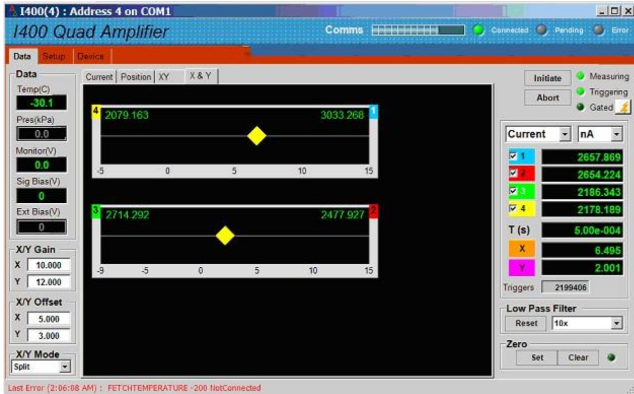
Figure 40. Independent X and Y position data tab, compensation factors, X/Y gains and offsets applied.
