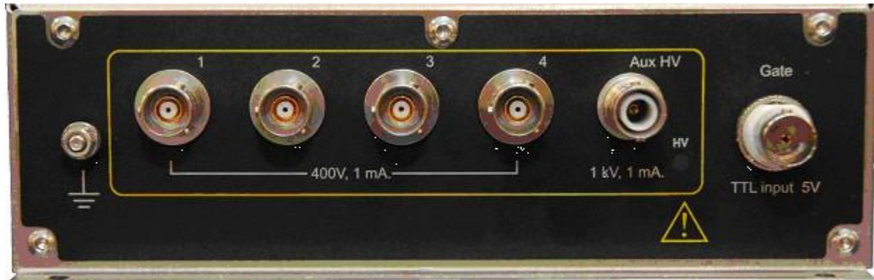
Figure 42. Front panel showing signal inputs, auxiliary HV output, gate input.
