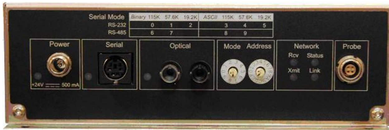
Figure 43. Rear panel power input, communications interfaces, temperature probe connector.
