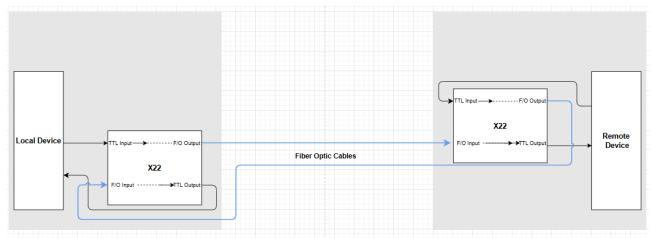
As shown above, place an X22 nearby the local device, using the shortest possible Coax cable to minimize EMI and signal loss. Bridge the gap between the local and remote devices with a fiber optic cable. Similarly, use a 2nd X22 at the opposite end to convert the signal back into TTL for the remote device. Return the signal output from the remote to local device using a 2nd fiber optic cable.
