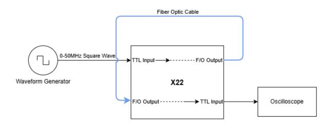
To test the capabilities of the X22, use a waveform generator on the TTL input, loop the fiber optic output to input, then readout on an oscilloscope. This can also be useful for determining if the cables used are functional. The most common issues are damaged or improperly terminated fiber optic cables.
