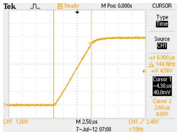
Figure 44. M10 analog output step without ramp rate limiting
