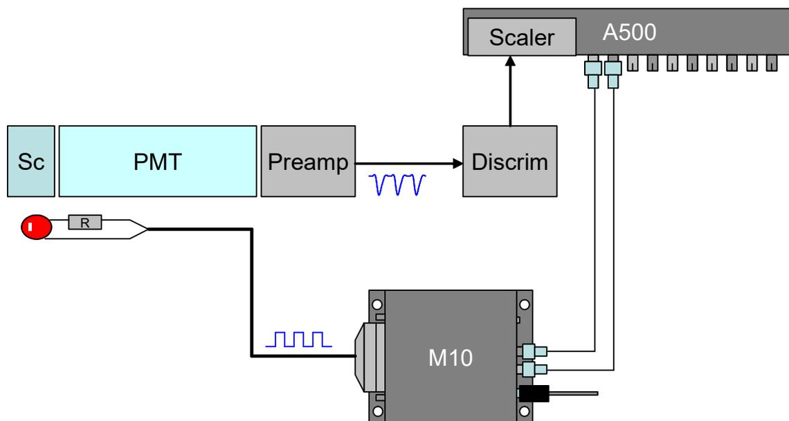
Figure 46. Use of the M10P to generate a pulse train for a pulser LED to test a pulse counting system.
