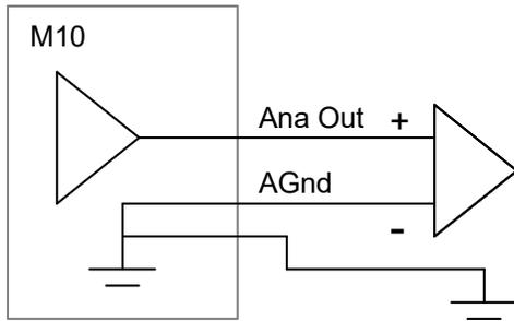
Figure 24. M10 connection to a differential analog voltage destination.
