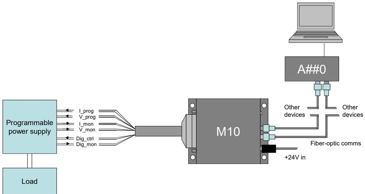
Figure 5. Schematic M10 installation for remote control of a power supply
