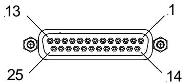
(External view on connector / solder side of mating plug)
