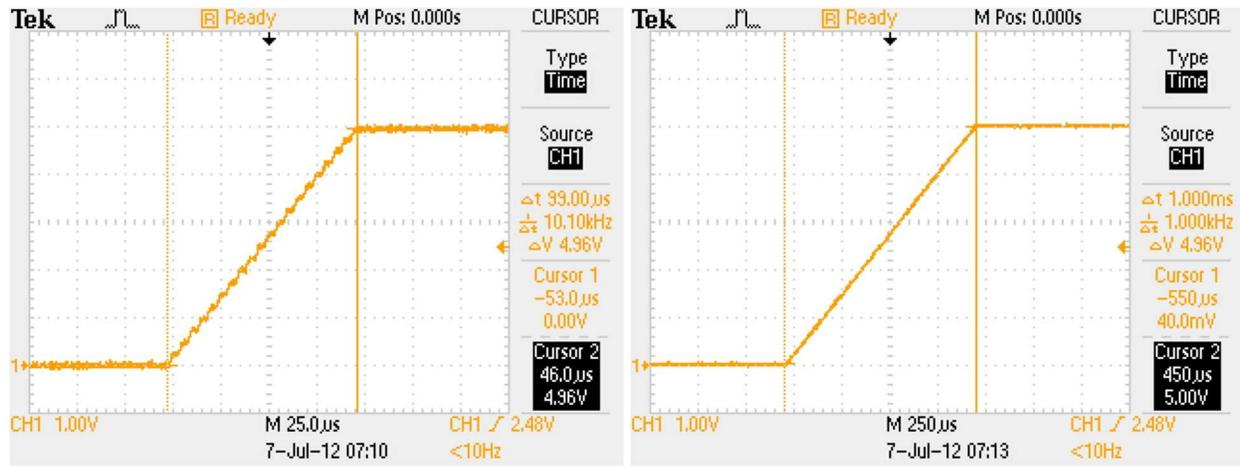
Figure 45. M10 analog output step with ramp rate limiting at 50000 V s<sup>-1</sup> (left) and 5000 V s<sup>-1</sup> (right)
