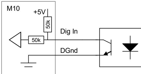
Figure 32. M10 digital input from an opto-coupler phototransistor.
