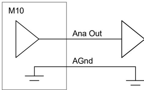
Figure 25. M10 connection to a single-ended analog voltage destination.
