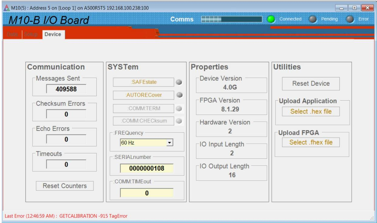
Figure 12. Device tab, showing firmware update utility controls.
