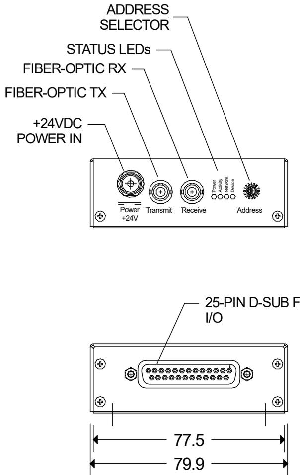
Figure 1. M10 chassis end panels. Dimensions mm.
