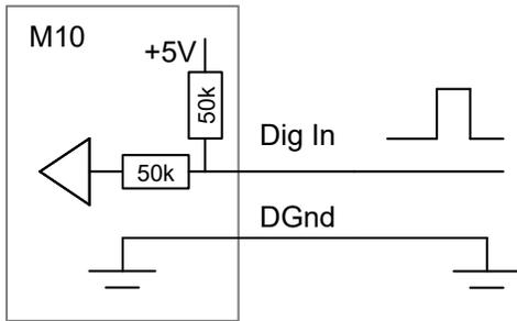
Figure 30. M10 digital input from a TTL source.
