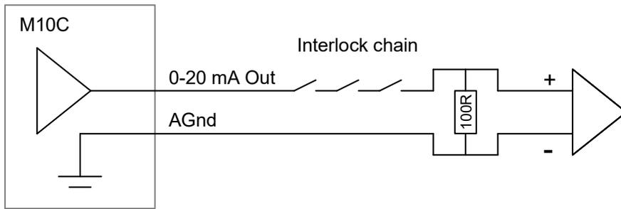
Figure 27. Analog current output showing external interlock chain.
