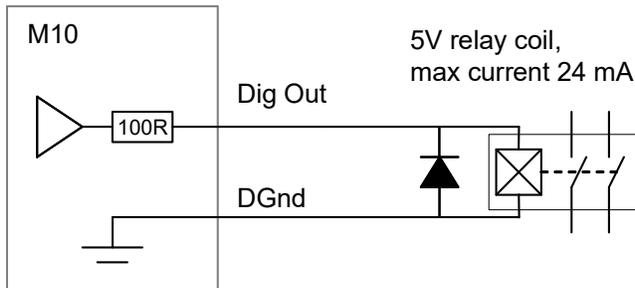
Figure 35. M10 digital output to relay solenoid.
